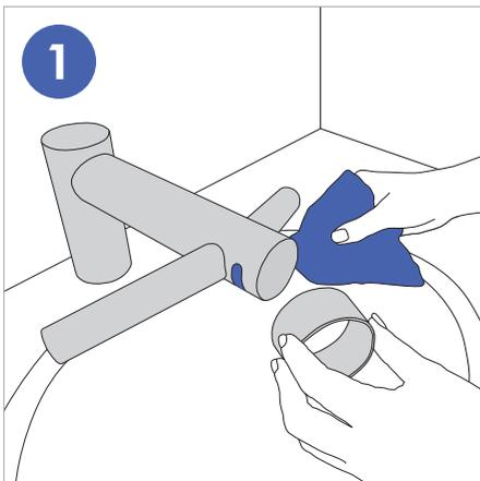
Wipe sensors using a soft cloth and non-abrasive cleaner then place cleaning cap over sensors to prevent activation.
